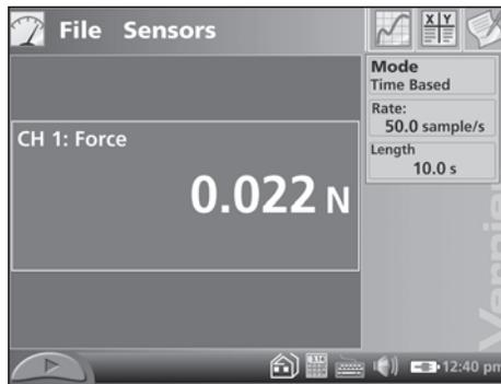
**3** Press the Collect button just below the LabQuest screen. Data collection begins, and a graph shows your data being plotted in real time.
