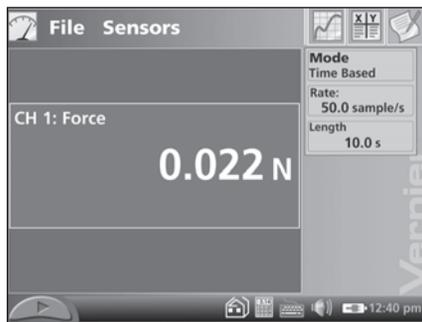
The Meter screen displays a digital meter for each sensor, the current mode, and data-collection parameters.
