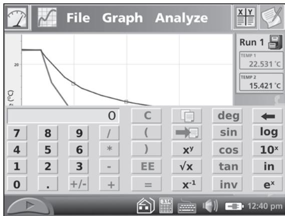
A **standard scientific calculator** is called by tapping the Calculator icon. The calculator uses algebraic notation. You can use this calculator at any time; to dismiss it, tap the Calculator icon again.
